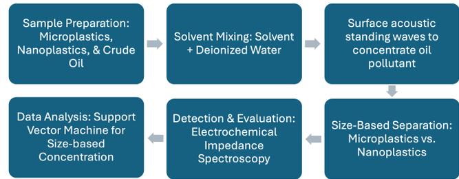
Fig. 1: Workflow for the sensor: sample preparation, dilution, oil pollutant separation, microplastic concentration and separation, plastic detection, and data analysis.
