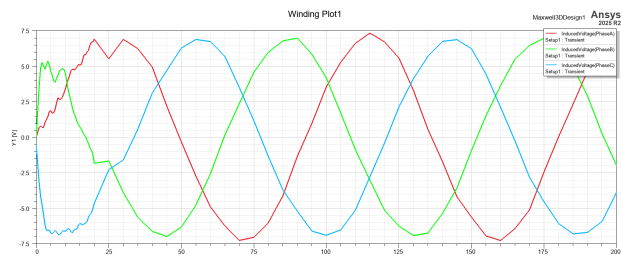
Fig. 11: Voltage induced across the three generator windings.
